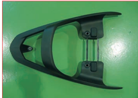
Glass Filled Polypropylene for "Pillion Handle" replacing Engg. Plastics
