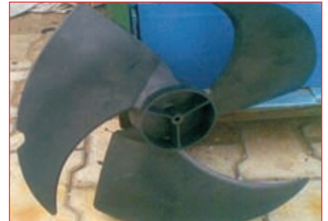
Glass Filled Polypropylene for AC Blower fan replacing Engg. Plastics
