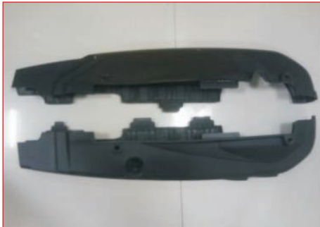
Polypropylene Two Wheeler Chain Cover replacing metal
